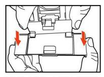
Next, pull the bottom portion of the accessory tool away from the lower clips.
