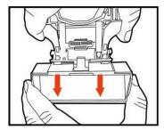
4. While the locking tab is held down, pull the top portion of the accessory tool away from the vehicle.
