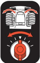
\* If vehicle pulls to the left or right during forward driving the Steering Trim may need to be adjusted. The Steering Trim is located on TOP of chassis under vehicle body, in between the front wheels.
